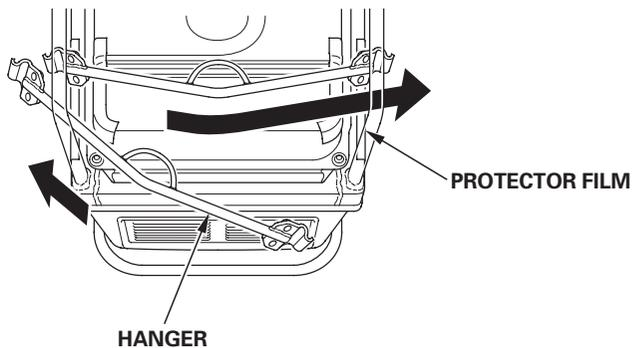
3. Slide the hanger along the frame pipe to align the center of the hanger with the recessed part on the rear side of the fuel tank. Install the hanger brackets on both ends of the hanger and tighten the  $8 \times 16$  mm flange bolts securely.
