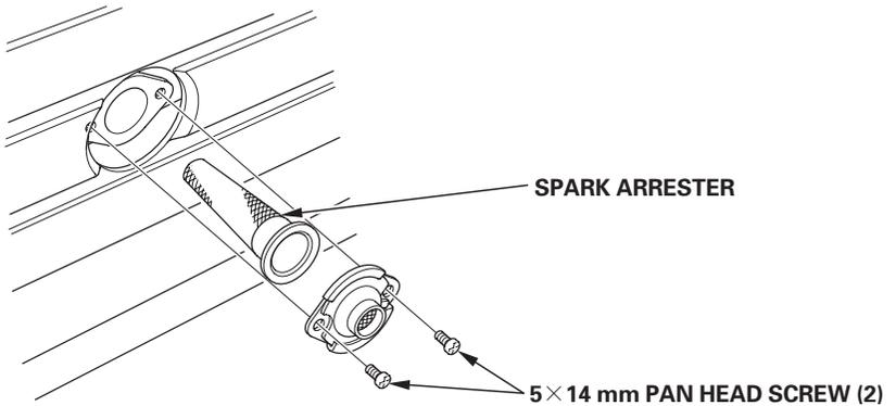
2. Use a brush to remove carbon deposits from the spark arrester screen.
