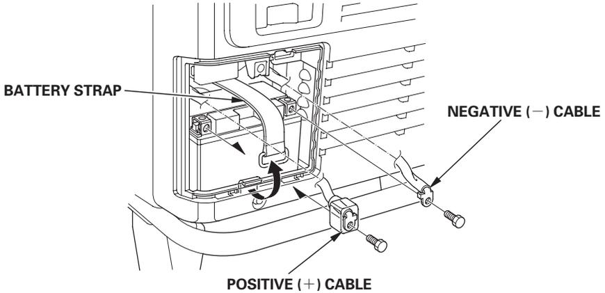
5. Remove the battery from the battery tray.
