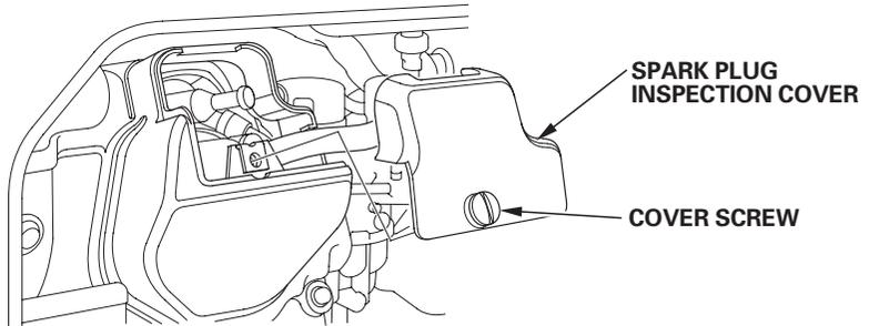
3. Disconnect the spark plug cap, and remove any dirt from around the spark plug area.
