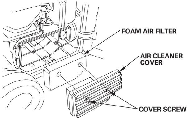
3. Remove the foam air filter from the air cleaner cover.
