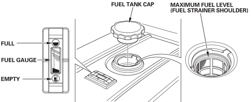
Refuel in a well-ventilated area before starting the engine. If the engine has been running, allow it to cool. Refuel carefully to avoid spilling fuel. Do not fill the fuel tank above the fuel strainer shoulder.
