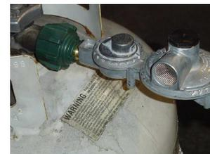
Ensure that all hoses, fittings and the regulator are properly protected from heat and accidental damage. Hoses can be burned or chaffed if routed improperly. Hoses are secured at the BRMC factory with tie down plastic straps to prevent chaffing. Be sure that all burner control valves on the grill are turned off (in the horizontal position). After connection is complete, check for leaks.
