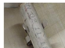
**i. IMPORTANT: Holes along the burner must be in the horizontal position for grill to work properly. Burners placed with holes in the vertical position will clog, not operate properly, and could create a fire hazard**
