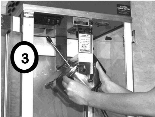
4. Insert the three prong kettle plug into the receptacle located on the inside of the machine on the underside of the ceiling of the unit, and twist gently clockwise to ensure a firm connection.
